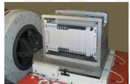
Fig.: Shock and vibration test to MIL 810G and IEC 61587-1, requirement classes DL2 and DL3
